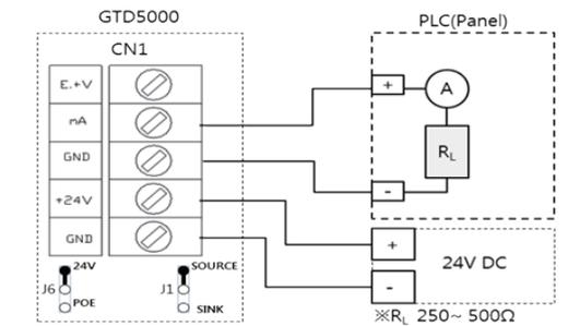
[Figure 7. 4~ 20mA Source Driver Configuration]
