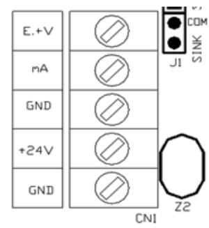
[Figure 6. CN1 Terminal Configuration]
