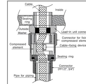
[Figure 17. High-Pressure Packing Type]
