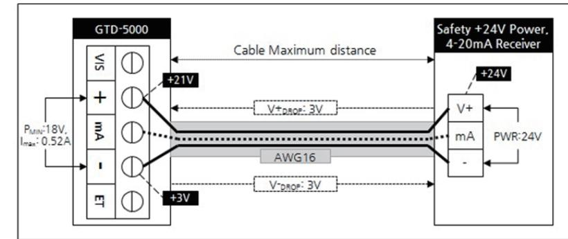
[Figure 13. GTD-5000 Installation Cable Length Calculation]
