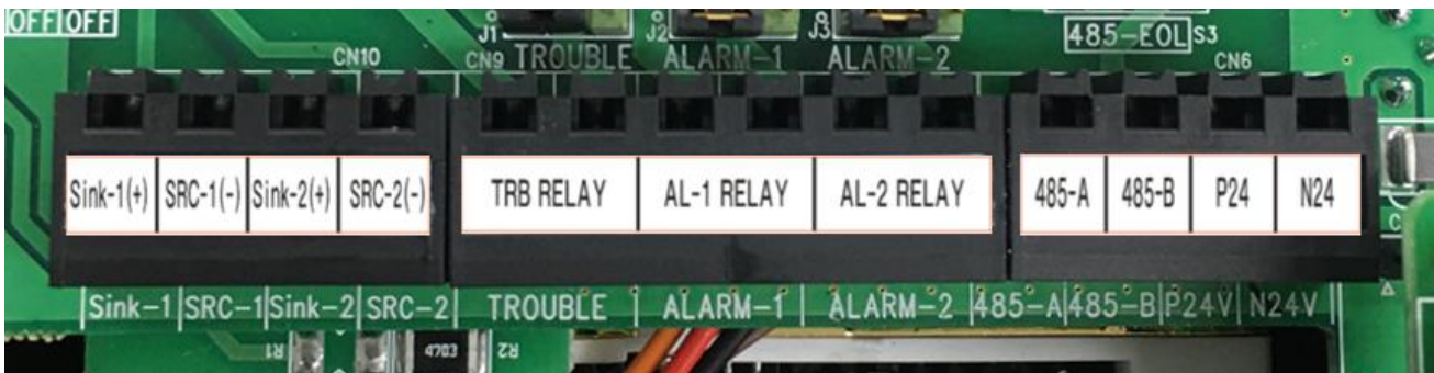
[Figure 9. Standard Terminal Layout]
