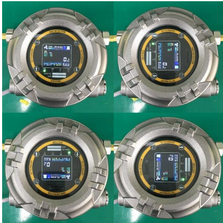
[Figure 7. Display Cover Turning]
